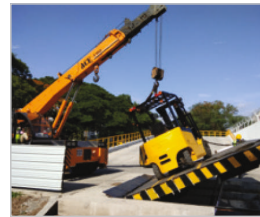
Forklift Stability as per ISO 22915-2
