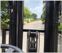
I-section, heavy duty and high visibility mast
