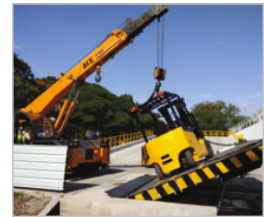
Forklift Stability as per ISO 22915-2
