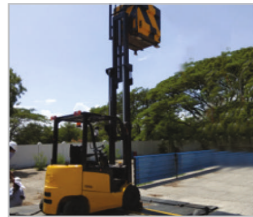
Forklift Stability as per ISO 22915-2
