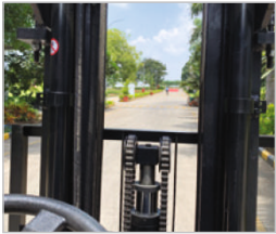
I-section, heavy duty and high visibility mast
