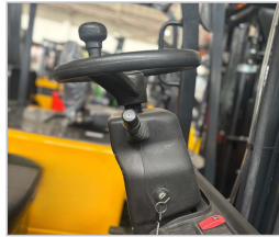
Tiltable Steering for better operator comfort to show 3D tiltable
